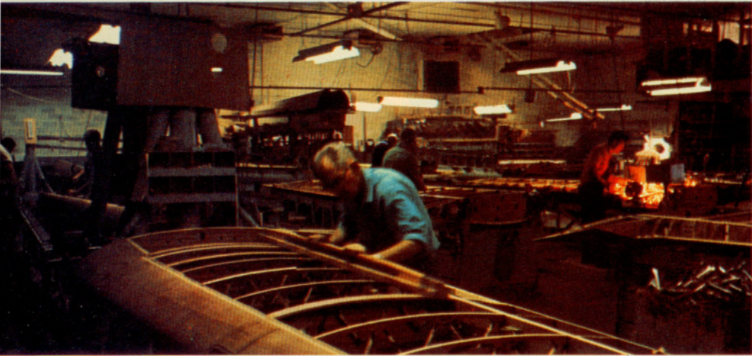
At Bellanca's factory in Alexandria, Minn., a workman toils over a Viking wooden wing. All photos by the author except as noted
